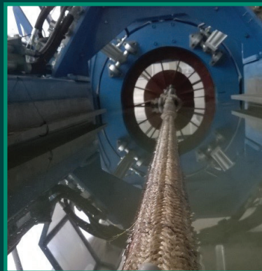
Figure 3: Submerged testing of the Exeter Tether mooring component using optical tracking equipment.
