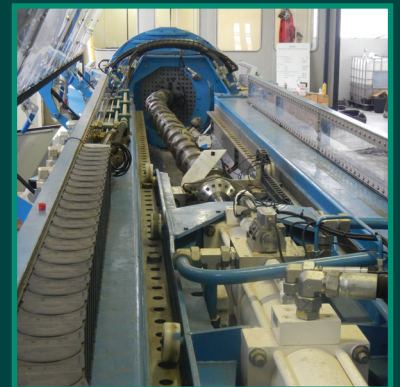
Figure 4: Fatigue testing of CNPL subsea-cable bend-restrictor.
