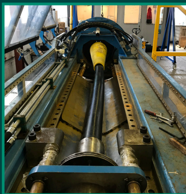
Figure 6: Cable and Bend stiffener testing.
