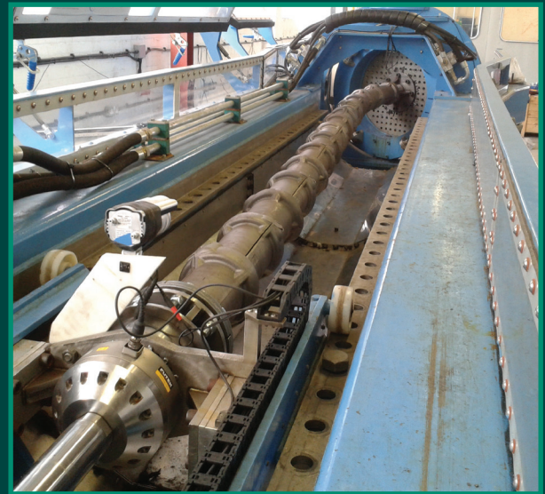
Figure 13: Cyclic bending test of CPNL bend [7].
