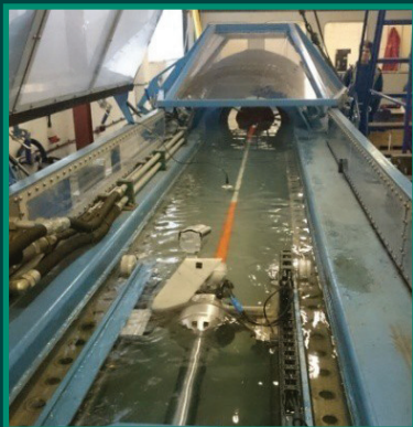
Figure 2: Submerged testing of Lankhorst mooring rope.
